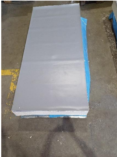
Picture 52 Picture 35 Rhenofol CV, Polyester reinforced PVC roof sheet specimen 3
