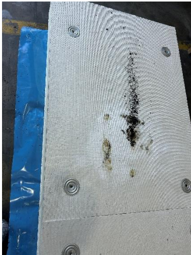
Picture 31 BarrierSheet after testing
