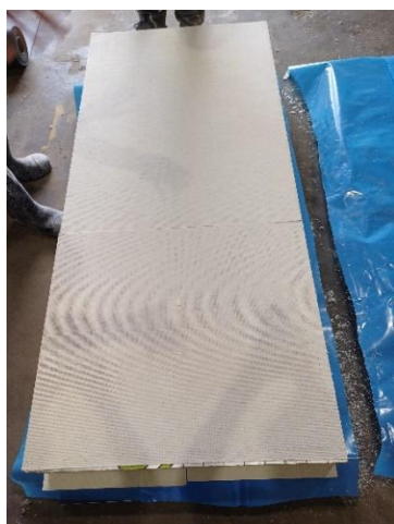
Picture 44 AllShield BarrierSheet above insulation specimen 1
