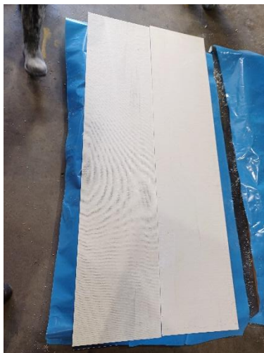
Picture 42 AllShield BarrierSheet under insulation specimen 1
