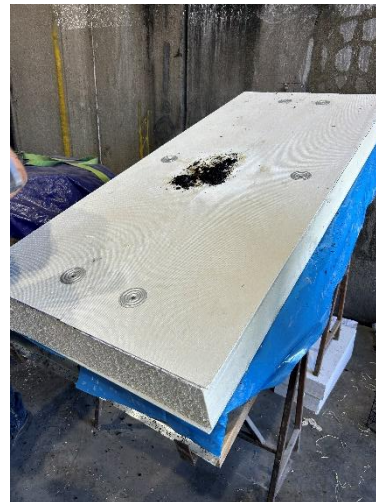
Picture 34 BarrierSheet after testing
