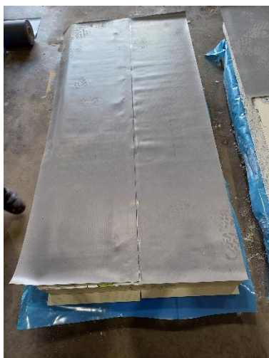
Picture 46 Rhenofol CV, Polyester reinforced PVC roof sheet specimen 1
