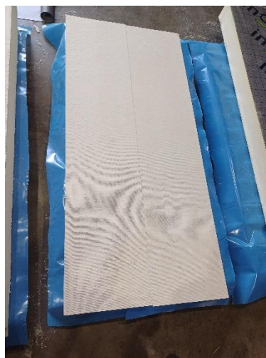
Picture 47 AllShield BarrierSheet under insulation specimen 2
