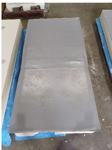
Picture 55 Rhenofol CV, Polyester reinforced PVC roof sheet specimen 2
