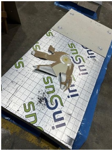
Picture 35 insulation after testing
