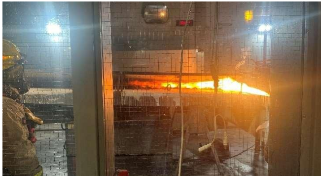
FM 4470 with AllShield Blue + PV (10min): Class 1
